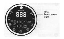
After replacing the filter, reset the filter replacement warning by pressing and holding the filter replacement button for 5 seconds.
